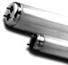
A T12 (top lamp) and a T8. The T12 measures twelve eighths of an inch or 1.5 inches in diameter; the T8, eight eighths of an inch or 1 inch in diameter. Pin spacing is the same for both lamps, facilitating replacement.
